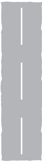
Hazard warning line (replaces a centre line or a lane line). An upright sign may indicate the nature of the hazard, such as a bend. The marking is used also on the approach to a junction
