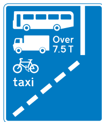
Near-side, with-flow bus lane ahead that can also be used by lorries, pedal cycles and taxis
