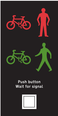
Near-side signals for Toucan crossing
